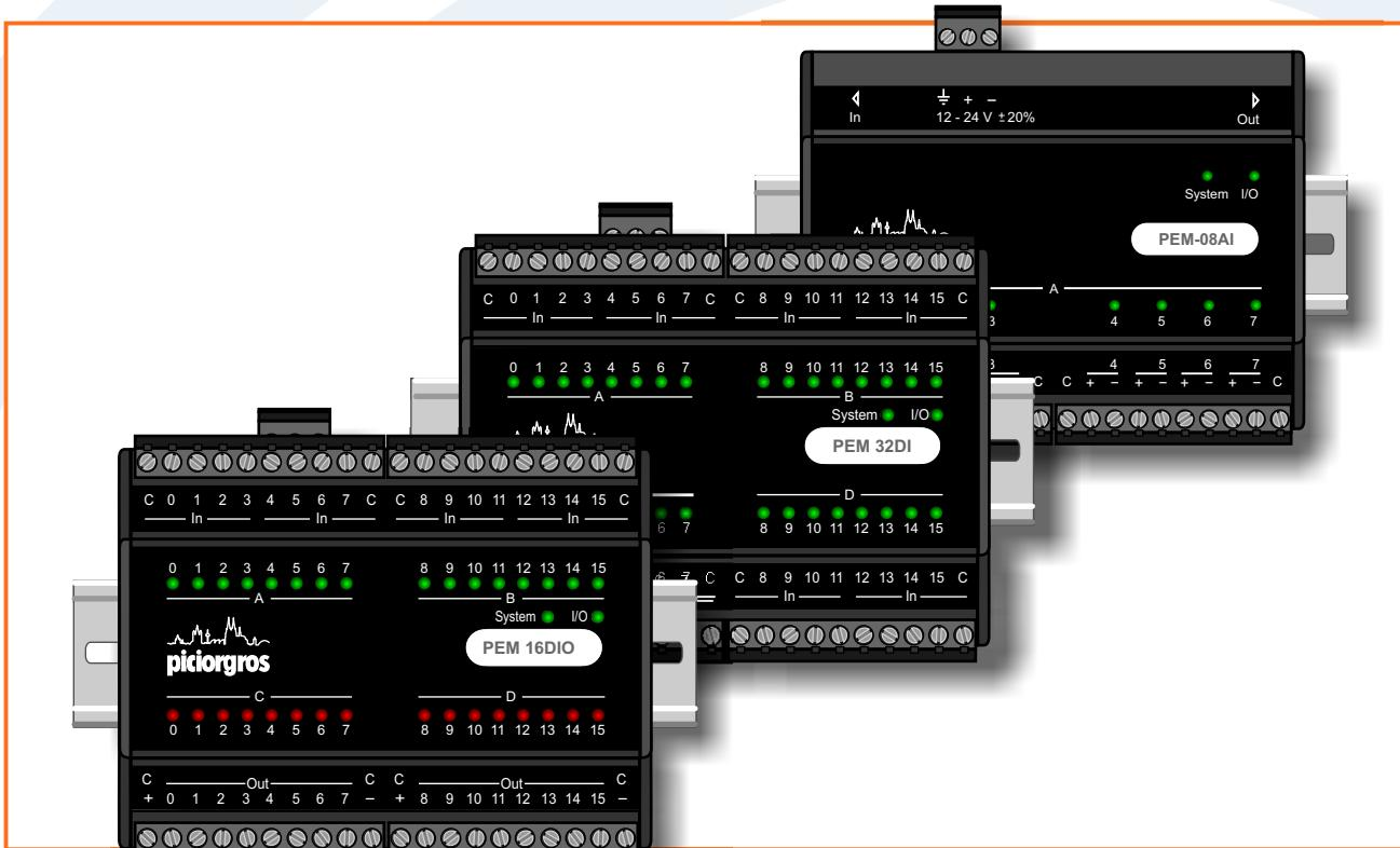
Piciorgros Radio RTU Modules each have an I/O expansion interface (Intel BitBus) through which up to 16 PEM I/O Expansion Modules can be bus-connected. With this, radio RTU stations can be configured with a large number of on-off inputs and outputs, analog inputs and outputs, and pulse inputs. On-off input and output states are indicated by LED lamps on the front face of each module.
